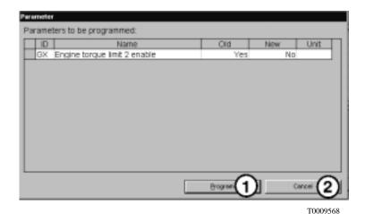
When a parameter value has been modified, the programming dialog appears to review and confirm the parameter changes that are to be carried out.
